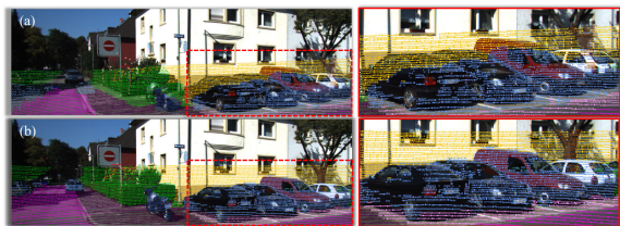
Fig. 9. Qualitative results of the SE-Calib in study area I. (a) Projection with the initial boresight parameters. (b) Projection with the optimized parameters.
